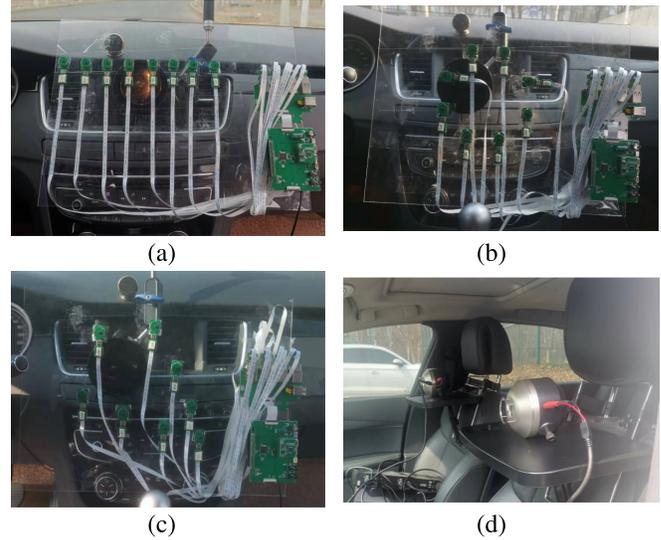
Fig. 9. Arrangement of the experiment equipment in a vehicle. (a) Eight-element uniform linear array, (b) eight-element uniform circular array, (c) eight-element designed MA, and (d) artificial mouths.
